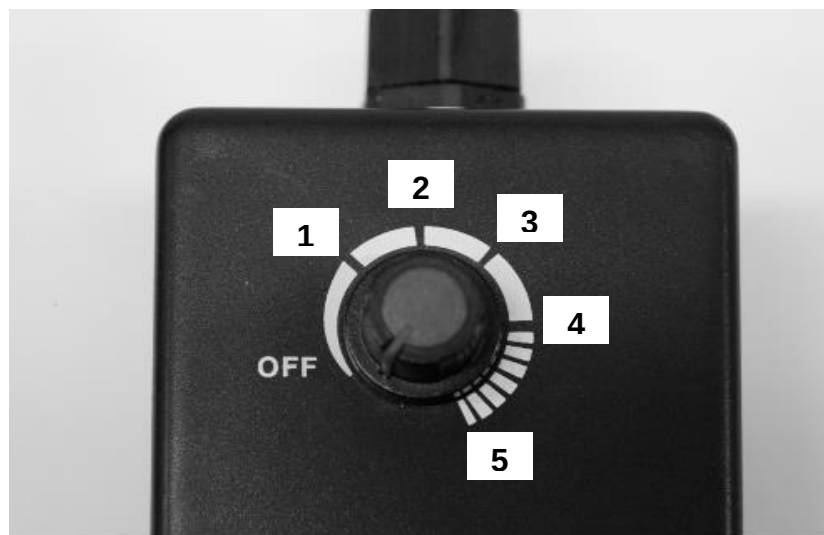
Fig. 1.3: Rotary switch for different speeds of air
